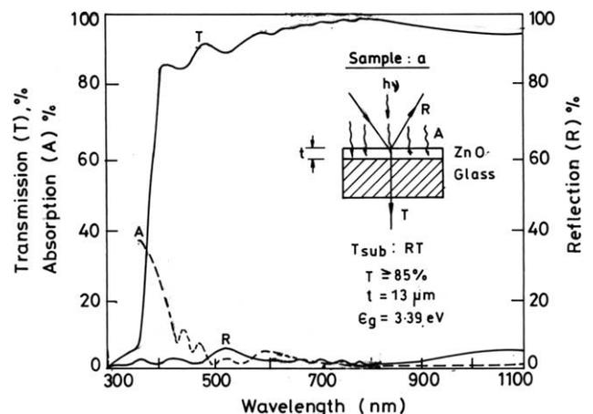
Fig. 1. Optical transmission, absorption and reflection spectra of ZnO thin films deposited at RT.
