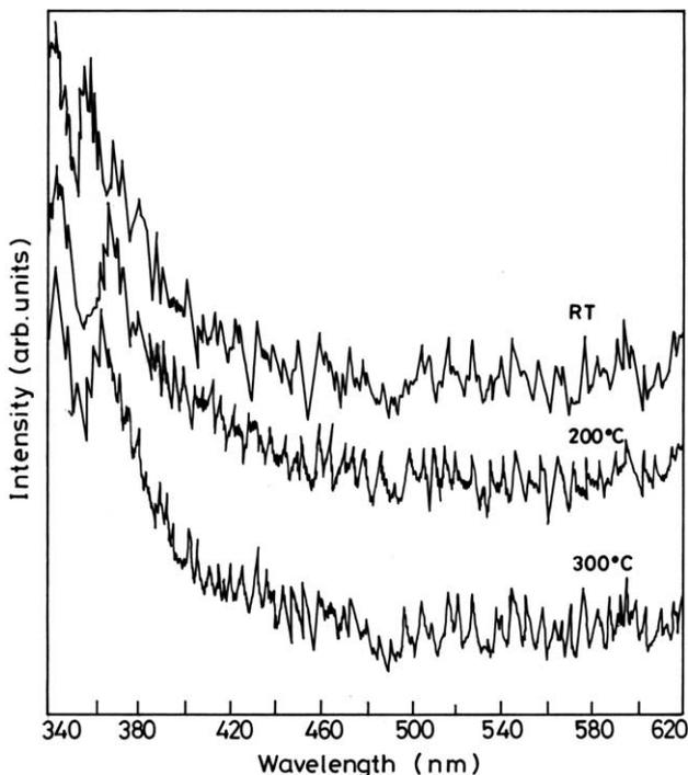
Fig. 7. Photoluminescence spectra of ZnO thin films deposited on float glass substrates at RT, 200 °C and 300 °C.
