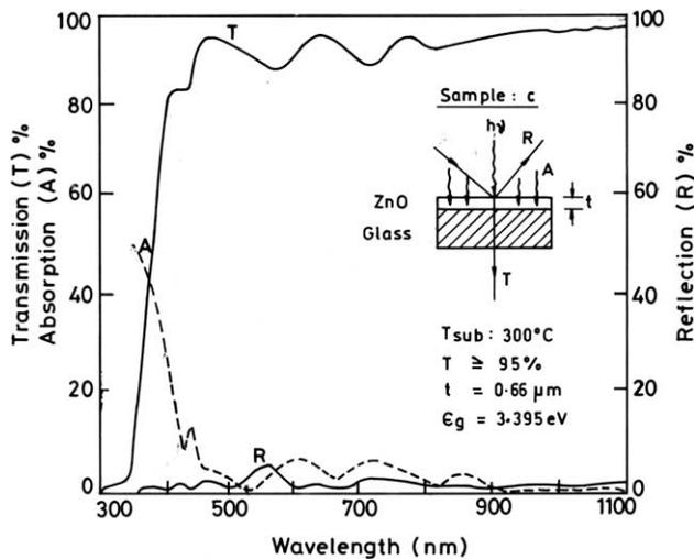
Fig. 3. Optical transmission, absorption and reflection spectra of ZnO thin films deposited at 300 °C.
