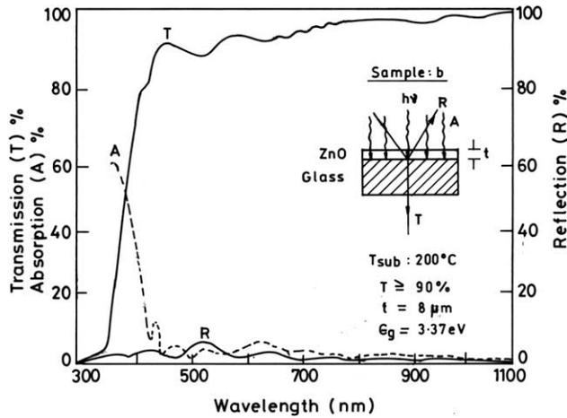
Fig. 2. Optical transmission, absorption and reflection spectra of ZnO thin films deposited at 200 °C.
