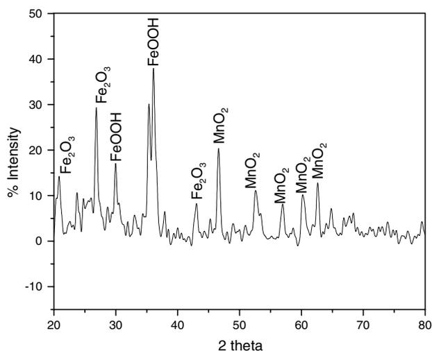
**Fig. 3** XRD pattern of corrosion product of experimental system, inoculated with Naphtha degrading bacteria (NDA)
