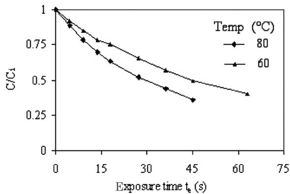
FIG. 3. Effect of temperature of heating medium on solids outlet moisture content. Material: Resin ( $d_p$ :  $530\mu\text{m}$ ); solids circulation rate:  $4.3\text{ kg m}^{-2}\text{s}^{-1}$ ; solids initial moisture content: 0.343.
