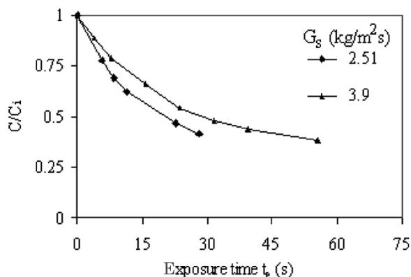
FIG. 4. Influence of solids circulation rate on solids outlet moisture content. Material: Resin ( $d_p$ :  $530\mu\text{m}$ ); solids initial moisture content: 0.343; temperature of the heating medium:  $80^\circ\text{C}$ ; flow rate of the heating medium:  $4.5\text{ m s}^{-1}$ .
