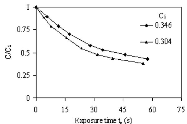
FIG. 6. Effect of initial moisture content of solids on drying rate, temperature of the heating medium:  $80^\circ\text{C}$ ; flow rate of the heating medium:  $4.5\text{ m s}^{-1}$ ; solids circulation rate:  $4.3\text{ kg m}^{-2}\text{s}^{-1}$ .
