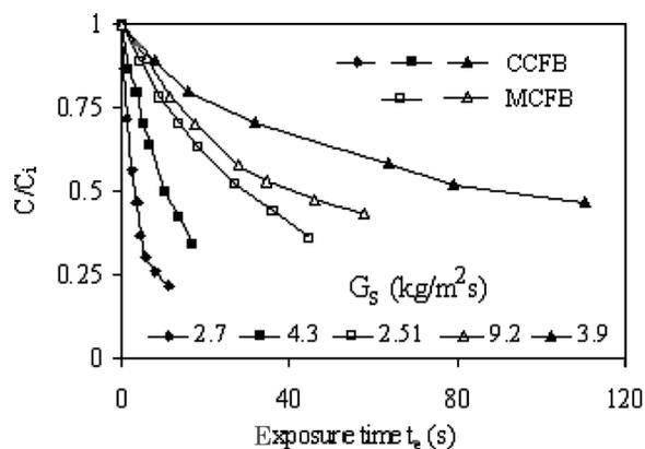
FIG. 7. Comparison of the drying kinetics in conventional circulating fluidized bed with circulating fluidized bed internals. Material: Resin ( $d_p$ : 530  $\mu\text{m}$ ); initial moisture content of solids: 0.343; temperature of heating medium: 80°C; flow rate of the heating medium: 4.5  $\text{ms}^{-1}$ .
