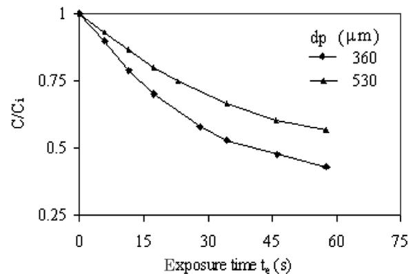
FIG. 5. Effect of particle size on solids outlet moisture content, initial solids moisture content: 0.348; temperature of the heating medium:  $80^\circ\text{C}$ ; flow rate of the heating medium:  $4.5\text{ m s}^{-1}$ ; solids circulation rate:  $3.9\text{ kg m}^{-2}\text{s}^{-1}$ .
