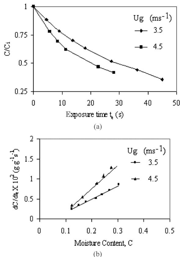
Fig. 2. Variation of (a) solids moisture content with drying time, (b) drying rate with moisture content. Material: Resin ( $d_p$ : 530  $\mu\text{m}$ ); initial moisture content of solids: 0.343; temperature of heating medium:  $80^\circ\text{C}$ ; solids circulation rate:  $2.51 \text{ kg m}^{-2}\text{s}^{-1}$ .
