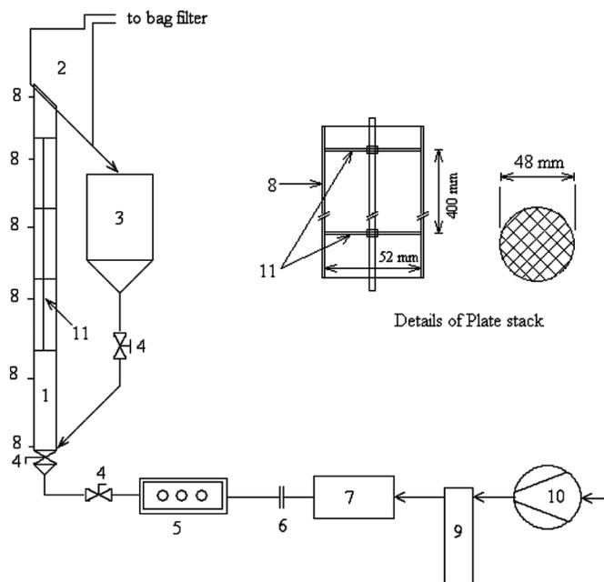
FIG. 1. Schematic diagram of the experimental setup: (1) test section, (2) gas–solids separator, (3) solids hopper, (4) control valve, (5) air heater, (6) flow meter, (7) surge tank, (8) pressure taps, (9) silica bed, (10) air blower, (11) plate stack.
