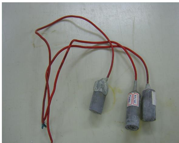
Fig. 2. Photograph for MnO<sub>2</sub> sensor.
