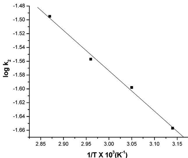
**Figure 6.** Plot of  $\log k_2$  and  $1/T$ . Conditions, electrolyte pH 6.5; concentration of phosphate,  $20 \text{ mg}\cdot\text{P/L}$ ; current density,  $0.05 \text{ A}\cdot\text{dm}^{-2}$ .
