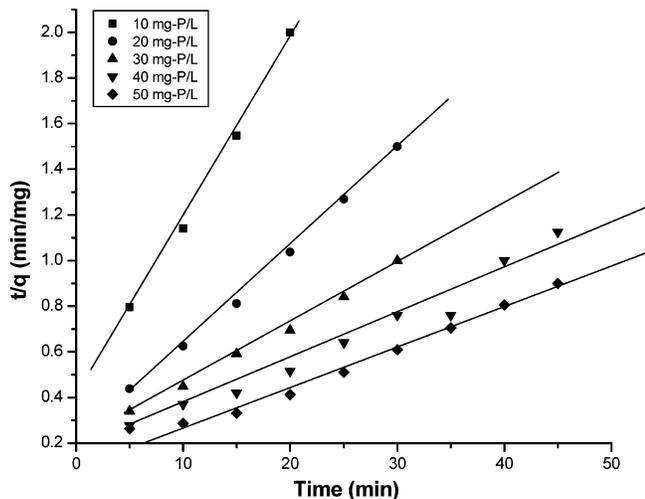
**Figure 4.** Second-order kinetic model plot of different concentrations of phosphate. Conditions, electrolyte pH 6.5; electrolyte temperature, 305 K; current density, 0.05 A·dm<sup>-2</sup>.
