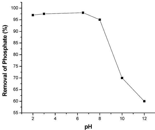
**Figure 3.** Effect of pH on the removal of phosphate. Conditions, concentration of phosphate, 100 mg·P/L; current density, 0.05 A·dm<sup>-2</sup>; agitation time, 60 min; electrolyte temperature, 305 K.
