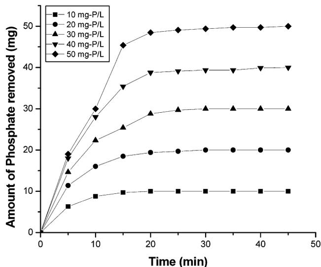
**Figure 2.** Effect of agitation time and initial phosphate concentration on the amount of phosphate adsorbed. Conditions, electrolyte pH 6.5; electrolyte temperature, 305 K; current density, 0.05 A·dm<sup>-2</sup>.
