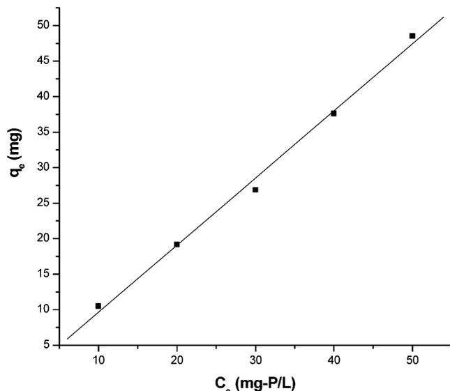
**Figure 5.** Langmuir plot ( $q_e$  vs  $C_e$ ). Conditions, electrolyte pH 6.5; electrolyte temperature, 305 K; current density,  $0.05 \text{ A}\cdot\text{dm}^{-2}$ .
