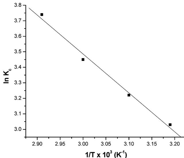
**Figure 7.** Plot of  $\ln K_c$  and  $1/T$ . Conditions, electrolyte pH 6.5; concentration of phosphate,  $20 \text{ mg}\cdot\text{P/L}$ ; current density,  $0.05 \text{ A}\cdot\text{dm}^{-2}$ .
