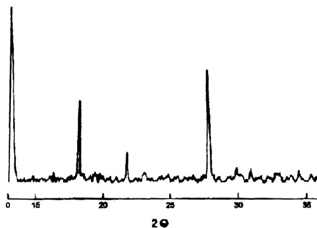
**Figure 8.** XRD diffractogram of electrocoagulation byproduct.
