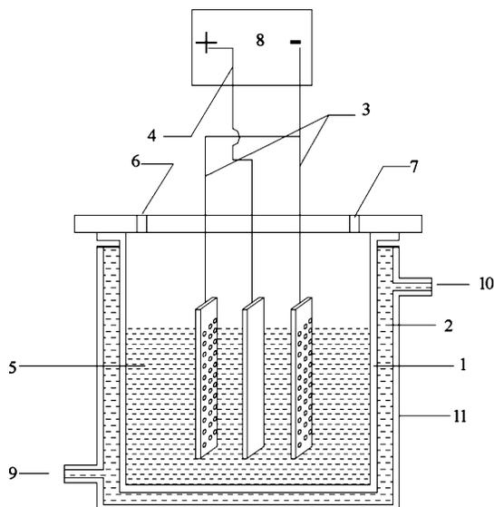
**Figure 1.** Laboratory scale cell assembly, (1) cell; (2) thermostatic water; (3) stainless steel cathode; (4) anode; (5) electrolyte; (6) and (7) holes to introduce pH sensor and thermometer; (8) dc source; (9) inlet of thermostatic water; (10) outlet of thermostatic water; and (11) thermostat.
