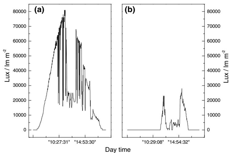
**Fig. 4** Typical discharge data on (a) a clear day and (b) a cloudy day for various type of lead-acid batteries employed during the present solar-lighting application study
