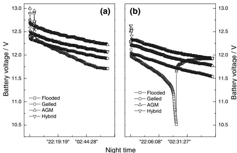
During the field performance test of the batteries for the stand-alone solar-lighting application, end-of-charge (EoC) voltage, end-of-discharge (EoD) voltage data and variation in peak-voltages obtained for hybrid VRLA, AGM VRLA,
