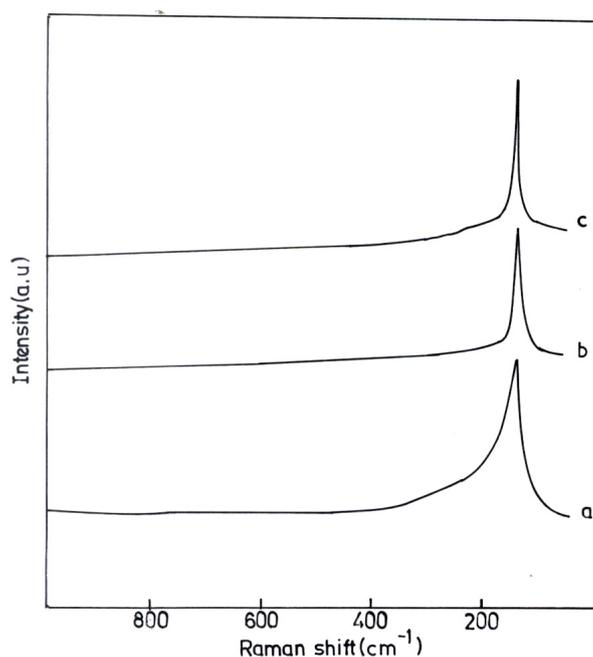
Fig.3. Raman spectra of PbSe films sintered at different Temperatures (a) 400°C (b) 450°C (c) 500°C
