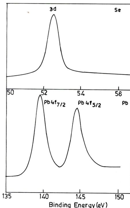
Fig. 2. XPS spectra of PbSe films sintered at 500°C
