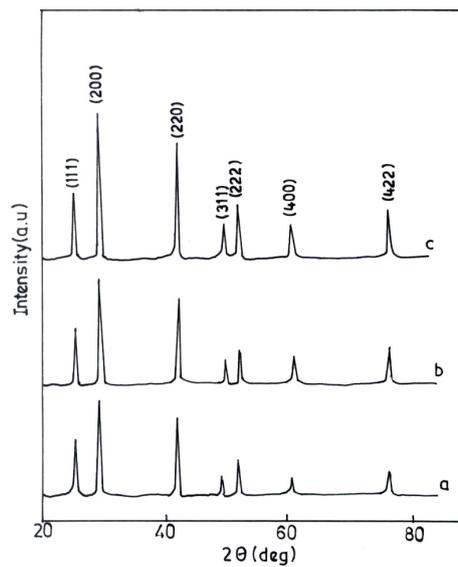
Fig. 1. X-ray Diffraction pattern of PbSe films sintered at different Temperatures (a) 400°C (b) 450°C (c) 500°C.
