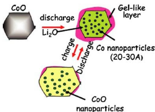
Fig. 1 Conversion mechanism in  $Co_3O_4$  (courtesy of Hu et al. [4])
