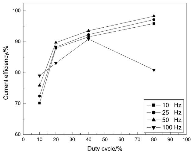
4 Effect of pulse duty cycle at various frequencies on current efficiency of copper deposit at 50°C
