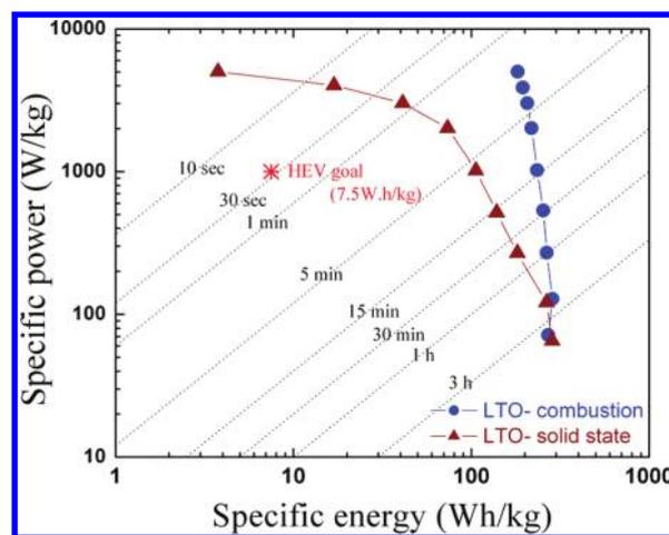
**Figure 8.** Ragone plot comparing the performance of  $\text{Li}_4\text{Ti}_5\text{O}_{12}$  prepared by (-●-) combustion method and (-▲-) solid-state method when paired with metallic lithium; (\*) DOE benchmark for HEVs.
