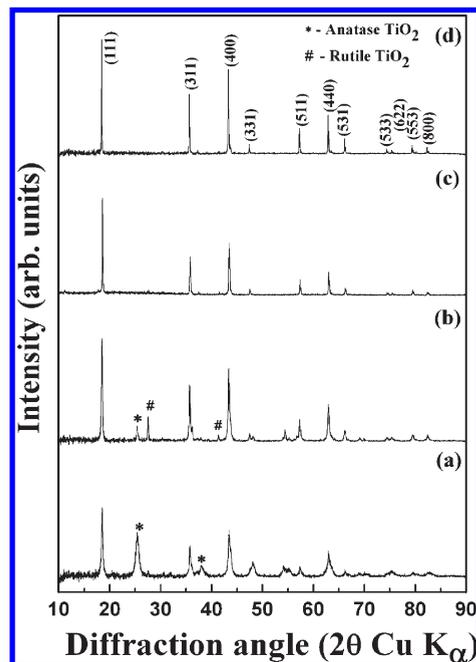
**Figure 2.** Powder XRD patterns for the products formed by the combustion of lithium and titanium nitrates with glycine at (a) 500 °C, (b) 700 °C, (c) 800 °C, and (d)  $\text{Li}_4\text{Ti}_5\text{O}_{12}$  prepared by solid-state method.
